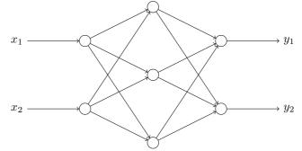
The left column of neurons (which receive the input signal  $\mathbf{x}$ ) is called the *input layer*. The right column of neurons which send out the response  $\mathbf{y}$  is called the *output layer*. The middle column of neurons is called the *hidden layer*. Each arrow connecting neurons carries its own weight-factor. Networks with one or more hidden layers are often called *deep neural networks*. Networks where the signal flow is always from left to right are called *feedforward* networks.
