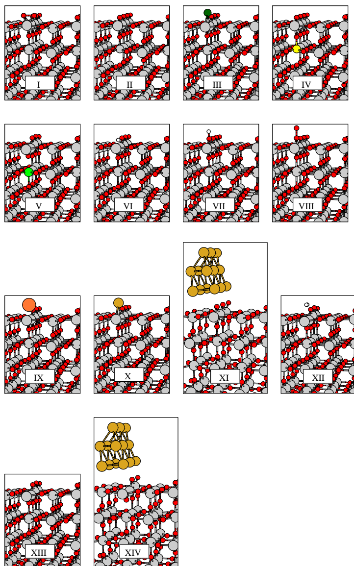
Figure 4.2: Ball-and-stick models of the different systems described in Table 4.1. XI and XIV were calculated in a p(3 \times 2) cell, all other systems were calculated in a c(4 \times 2) cell. I An O 2 lying in a vacancy. II The stoichiometric surface. III A Cl atom in a vacancy. IV A P atom in the stoichiometric surface. V A vacancy above an Al atom. VI An H in a vacancy. VII A OH in a vacancy. VIII O 2 upright in a vacancy. IX A Br atom in a vacancy. X An Au atom in a vacancy. XI A gold rod on the stoichiometric surface. XII H 2 in a vacancy. XIII Vacancy. XIV Gold rod on a vacancy.
