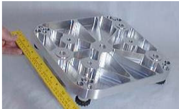
Figure 42 – Bottom view of the unanodized lightweight Base Plate
