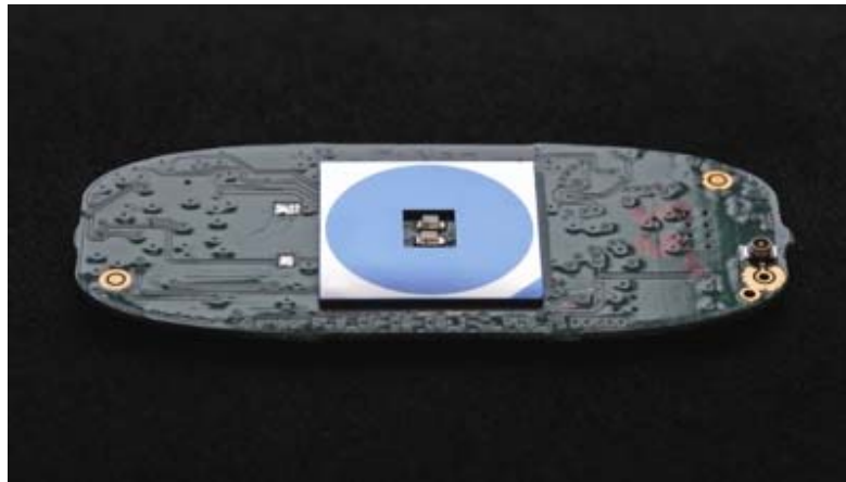
Figure 1. Silicon photodiode mounted on a printed circuit board. The photodiode has a hole in the center where two LED's are mounted..
