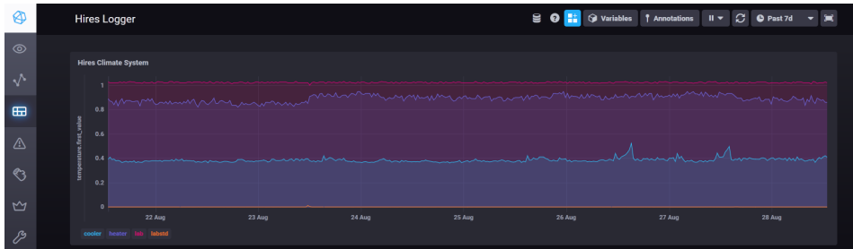
Figure C.1: A snapshot of the online Chronograph server, used for logging in our experiment. The graph displayed is the readout from the temperature sensors of the climate system over a period of one week. The vertical axis is not calibrated to temperature. The bottom line monitors the cooling part of the system, the middle one the heating part and the top one is the regulated temperature measured on the experiment table.
