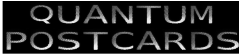
Figure 4.11: Example of a text writing by an time averaged laser beam controlled by an AOD.
