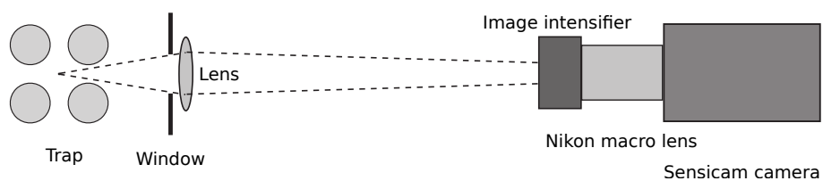
Figure 7.8: Schematic of the imaging system. In the setup, the camera is above the trap (vertical).
