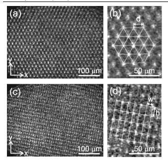
FIG. 4. Images of a cold ensemble of ~13 000 ions. (a) Visible hexagonal structures indicating a three-dimensional bcc structure. (b) Magnification of a section of (a). The side length *d* is found to be 17.2  $\mu$ m. (c) Visible rectangular structure likely indicating a slightly distorted fcc structure. (d) Magnification of a section of (c). Here,  $h = 15.2 \pm 0.5 \mu$ m and  $w = 9.71 \pm 0.2 \mu$ m, respectively.
