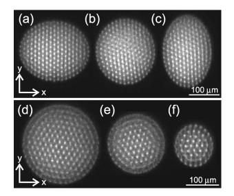
FIG. 2. Images of Coulomb crystals. The first column shows three crystal images of the same ensemble of ~2000 ion with the trap potentials being  $U_{\rm rf} = 500$  V and (a)  $U_{\rm end} = 27$  V, (b)  $U_{\rm end} = 33$  V, and (c)  $U_{\rm end} = 40$  V, respectively. The second column represents images near spherical crystals for the same trap potentials  $U_{\rm rf} = 400$  V and  $U_{\rm end} = 21$  V. The number of ions in the crystals is (d) 1700, (e) 770, and (f) 290.
