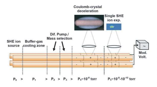
Fig. 1. Sketch of a possible experimental set-up for studies of sympathetically cooled SHE ions. The set-up consists of several sections, which are discussed in the text. Differential pumping will be very important since in the final step where, e.g., experiments using single SHE ions will take place, a pressure of at least  $10^{-9}$  torr is needed.
