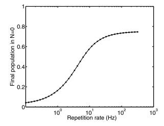
FIG. 4. Population in the rovibrational ground state of MgH<sup>+</sup> after 100 s of cooling as a function of the repetition rate of the pumping lasers. Each laser pulse saturates the transition it pumps.
