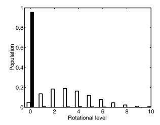
FIG. 5. Cooling of ArH<sup>+</sup> by the direct scheme. The unfilled columns represent the initial rotational populations corresponding to a thermal distribution at T = 300 K. The filled columns represent the population distribution after 50 s of cooling. See the text for details on the scheme, and the cooling parameters.
