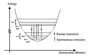
FIG. 1. Figure showing the intervibrational transitions needed for the Raman cooling scheme. A detailed explanation of the cooling principle is given in the text.
