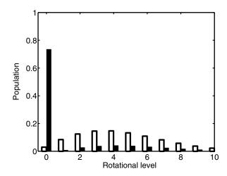
FIG. 2. Cooling of MgH $^+$  by the Raman scheme (see Fig. 1). The unfilled columns represent the initial rotational populations corresponding to a thermal distribution at  $T=300~\rm K$ . The filled columns represent the population distribution after 100 s of cooling. See the text for details on the cooling parameters.
