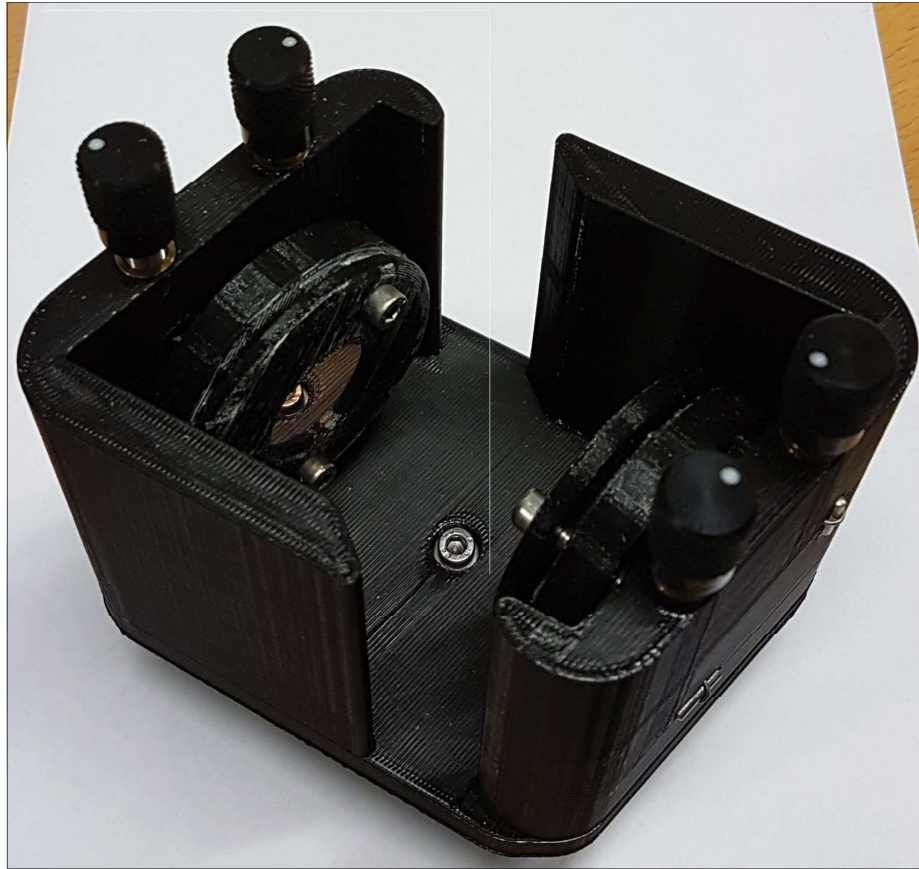
Figure 3.19: The first version of a compact double-mirror mount. It is a small box with two mirrors that can be used for optimisation.
