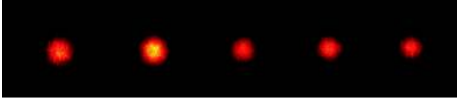
Figure 8.12: An example of microwave transfers in a one-dimensional optical lattice for atoms prepared in the F = 2 , m_F = +2 state. This figure shows the different m_F components— m_F = -2 (left) to m_F = +2 (right). The different m_F states are separated using the Stern Gerlach method (TOF is 10 ms). We can transfer almost all of the atoms into each of the different m_F states using a number of microwave sweeps. If we wait too long between the sweeps, we start to populate other m_F states—we assign this behavior to spin exchange collisions. This experiment was done together with Sune. Based on 010408 run 138.
