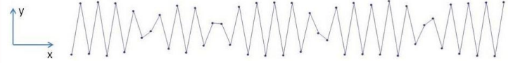
Fig. 3. Ion chain in a zigzag configuration exhibiting structural defects: the distribution of charges in two dimensions is mapped to a line for clarity. The solid line joining the ions serves as a guide to the eye. In the example reported, there are four defects.
